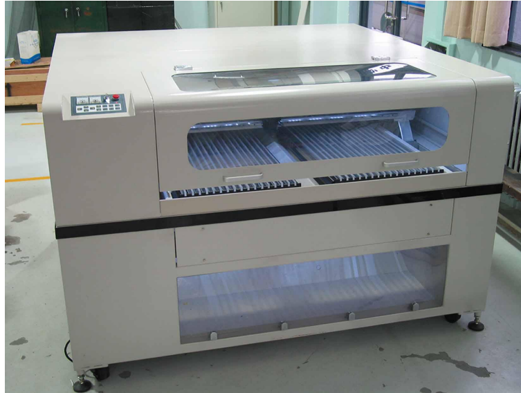
Plastic Mirror Laser Cutting
